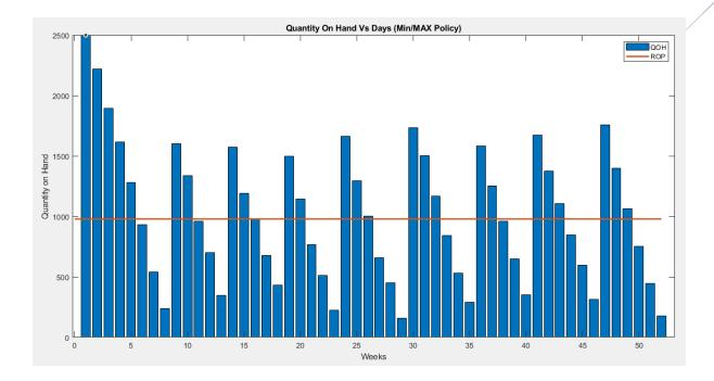
The graph shows the Quantity on hand vs weeks. Because the cycle time for making new inventory is 3 weeks, whenever inventory falls below the ROP, it will be ordered and restocked after 3 weeks. The graph shows no stockouts, but they could occur if there is an unexpectedly high demand. This is encountered, however, by taking a sufficient variance in weekly demand.
