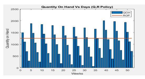
The Graph shows how the inventories are continuously reviewed and if it is found the quantity goes below it is ordered. Because the cycle time for making new inventory is 3 weeks, whenever inventory falls below the ROP, it will be ordered and restocked after 3 weeks. The graph shows no stockouts, but they could occur if there is an unexpectedly high demand. This is encountered, however, by taking a sufficient variance in weekly demand.
